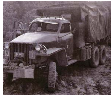
Studebaker 6x6 fitted with tipping body and canopy. Belonging to 1 Field Sqn, it was on loan to 2 Troop.
